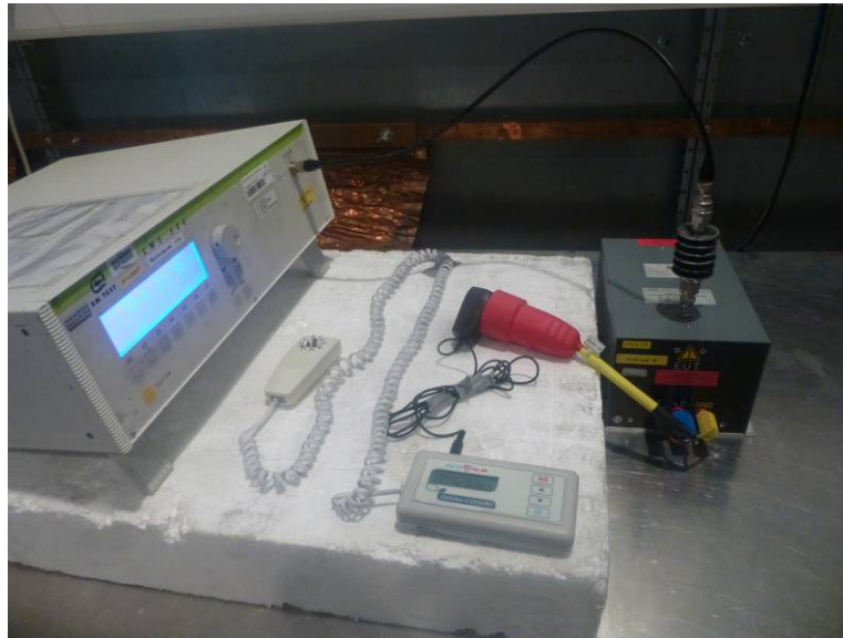
Figure 6-20: test setup for Injected currents, 0.15 MHz to 80 MHz
