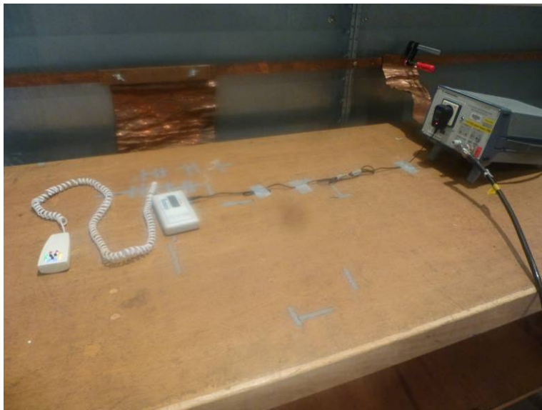
Figure 6-10: test setup for Discontinuous disturbance (Clicks)
