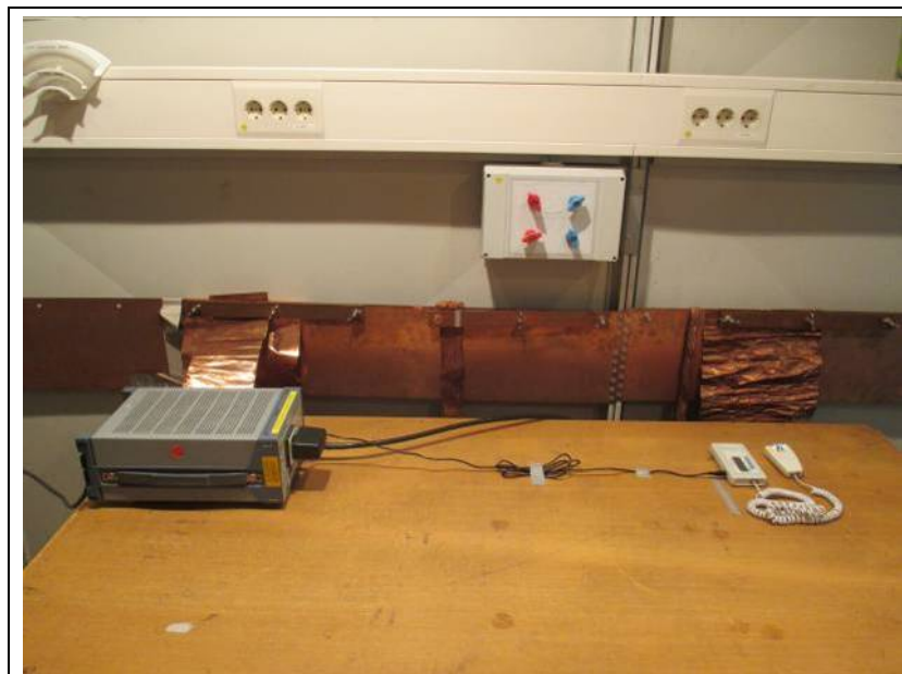
Figure 6-1: test setup for Continuous disturbance (terminal voltages)
