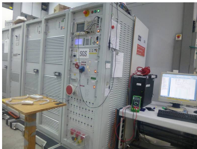
Figure 6-25: test setup for Voltage Dips and Interruptions
