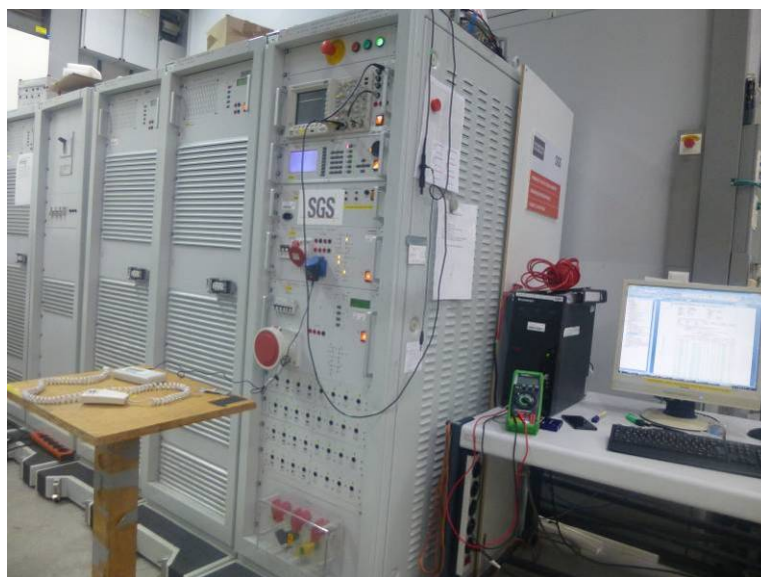
Figure 6-11: test setup for harmonic current emissions
