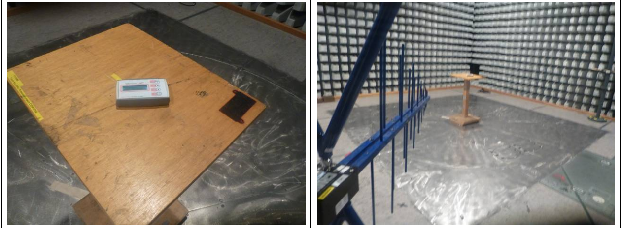
Figure 6-4: test setup for Radiated disturbances 30 MHz to 1000 MHz
